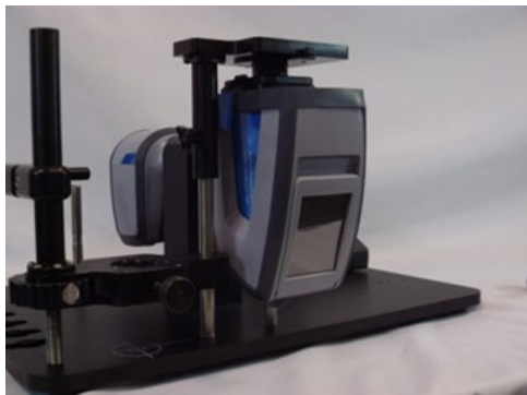
Figure 10 Installing the instrument in the stand
