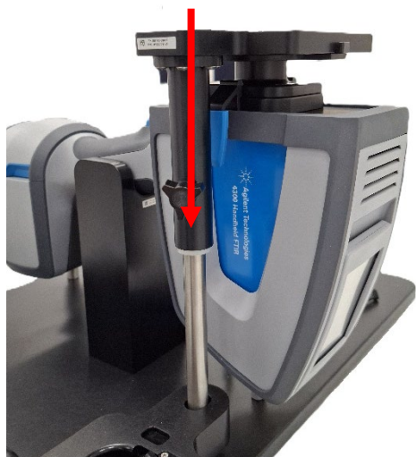
Figure 6 4300 Handheld FTIR mounted on the stand and sliding the ATR stage down the support rod
